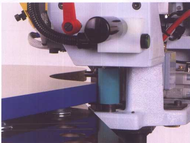
Quick change-over to a stationary edge bander
