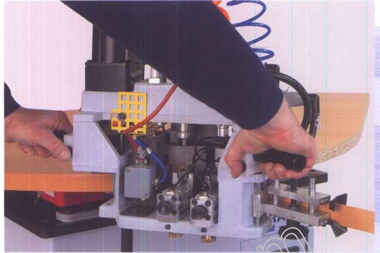
Freely moving gluing unit
