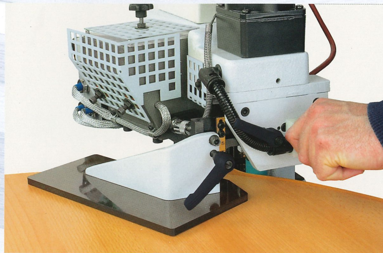
Guidance of the gluing unit by means of a height adjustable guiding plate
