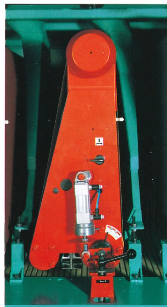
Combi-sanding head with automatic positioning of contact roller (option) and abrasive belt grit size compensation.
