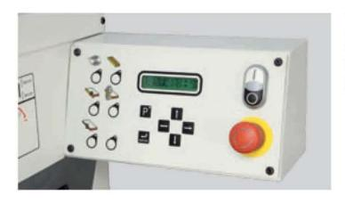
Control panel Control panel positioned at the machine's infeed in an ergonomical
