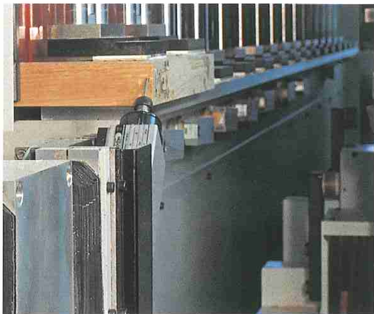
Incisore anti-scheggia a tre assi Cutting unit with anti-splintering device with 3 axes
