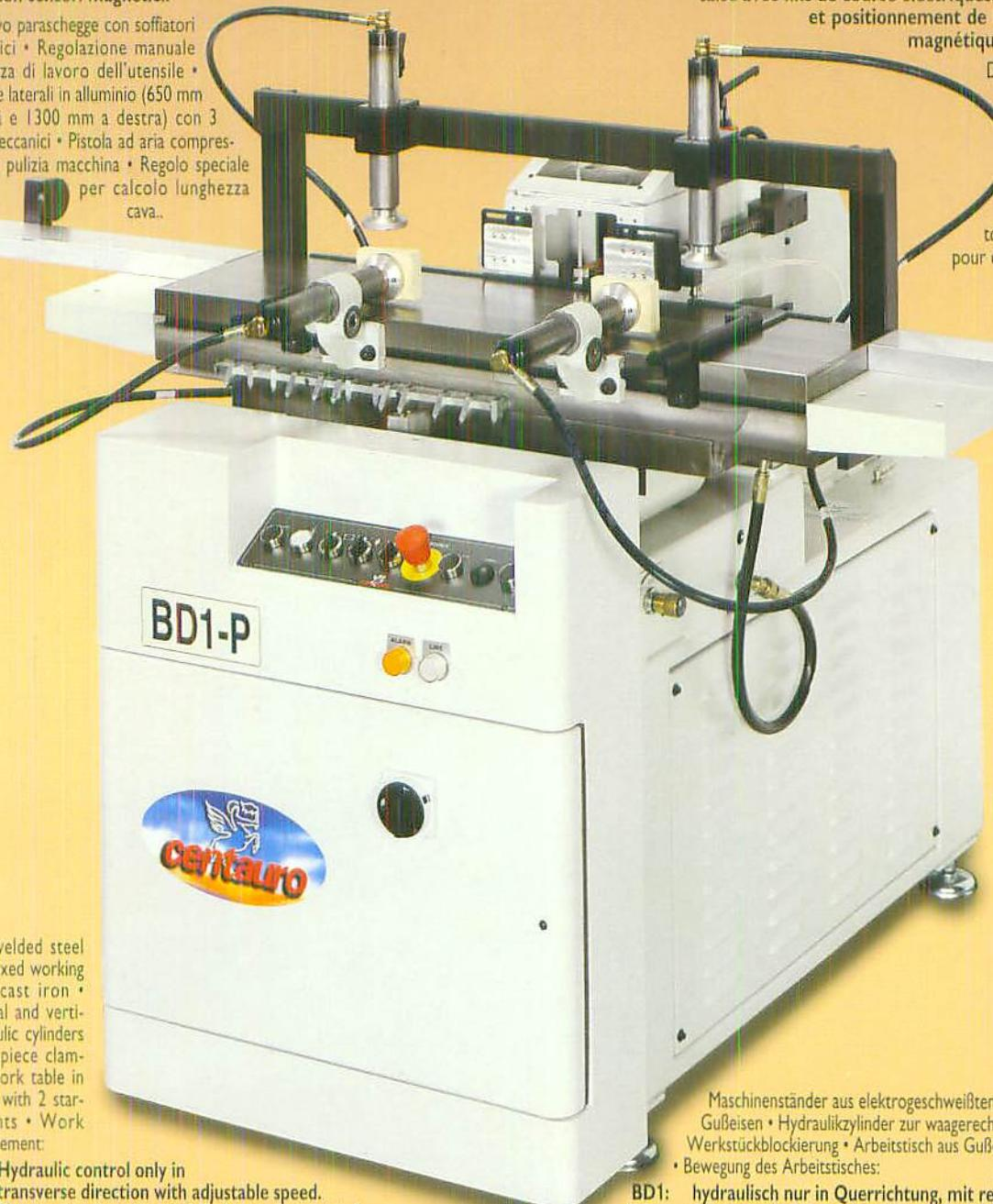
Electro-welded steel frame • Fixed working head in cast iron • Horizontal and vertical hydraulic cylinders for workpiece clamping • Work table in cast iron with 2 starting points • Work table movement:
