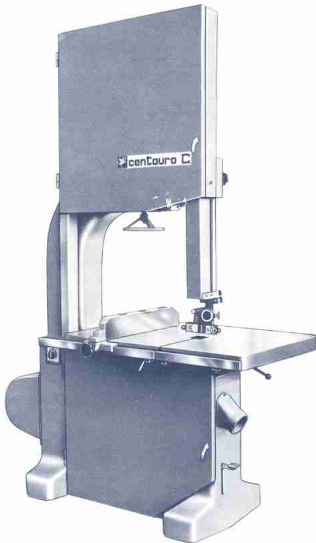
Art. 2218 Band saw classic - Mod. "CL900" - cast-iron table - wheels full
