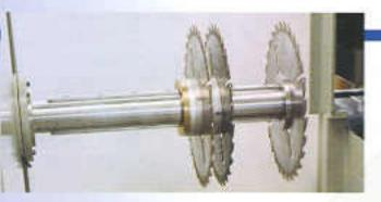
The surface treatment of the spindle ensures perfect running of the moving blade and long working life
