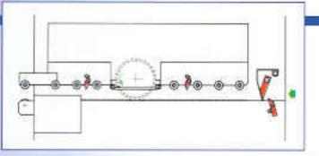
TOP ROLLERS GROUP raised automatically, with 8 independent hold-down rolls. The splinterproof system consists of steel fingers distributed on 3 top rows (one of which acting as splinterproof and the other two as anti-kickback) and one bottom row.
