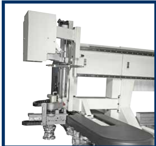
The MACH 5 device in only five seconds replaces the tool drastically reducing down-times.
