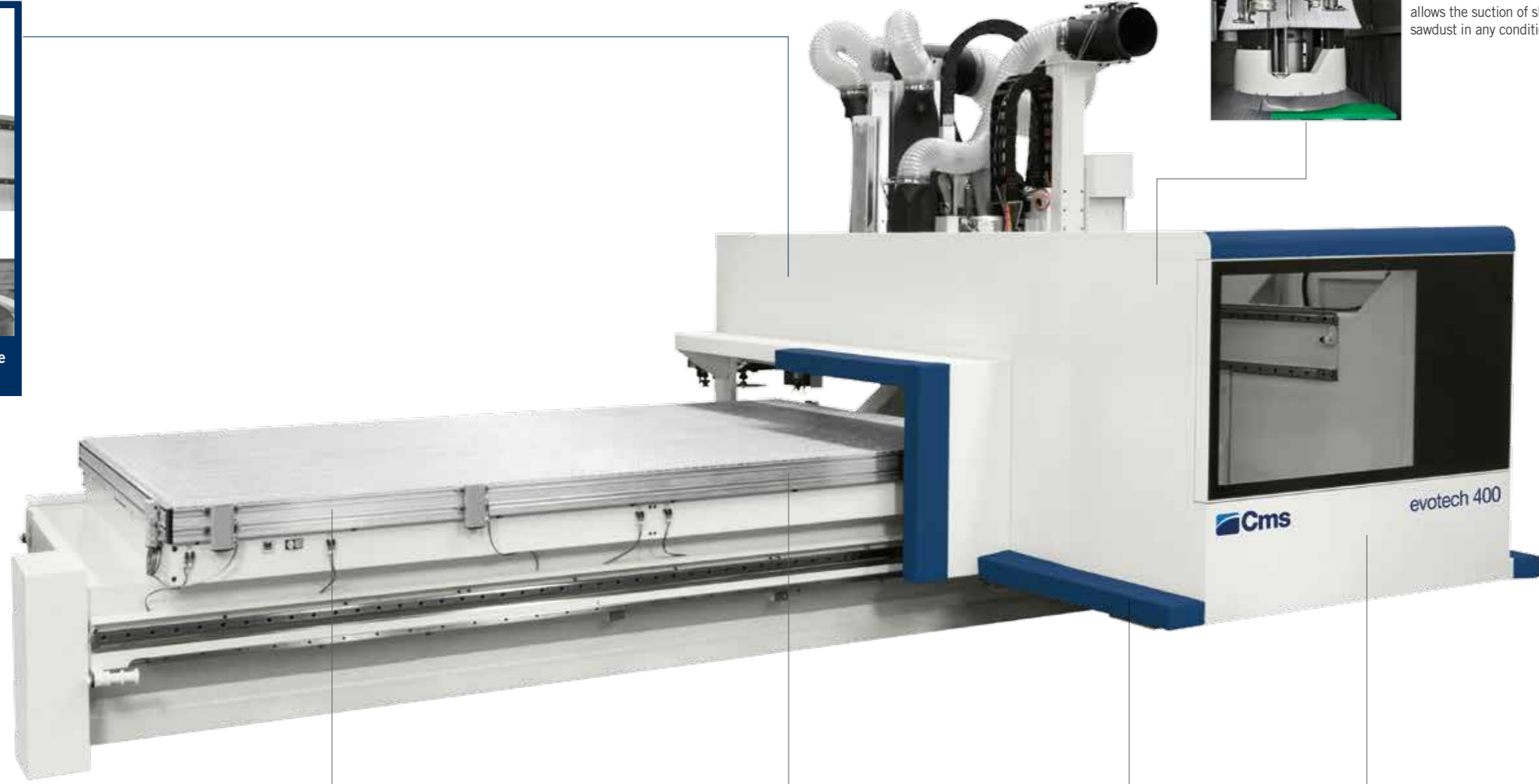
Guaranteed accuracy of the 5-axis with the RTCP setting (Rotation Tool Center Point system) that automatically re-adjust the machining head parameters through a self-calibration system and a software function available on the machine.
