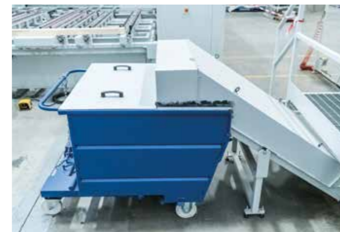
CHIP CONVEYOR Easy removal of scraps and dust
