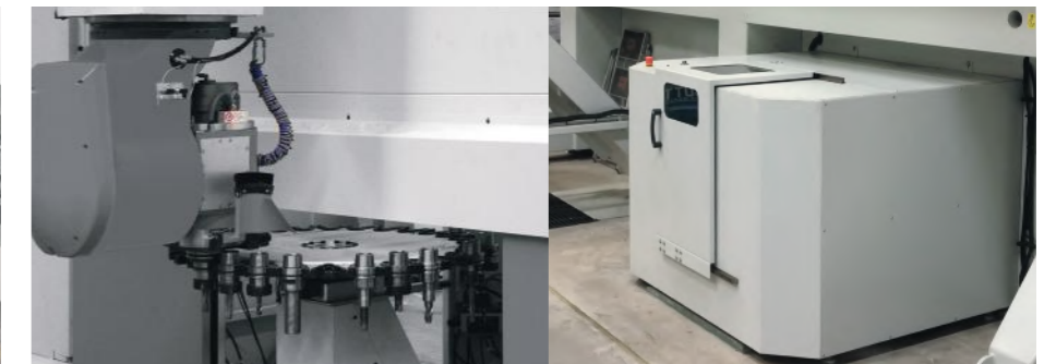
30 stations tool changer magazine internal and exterior view
