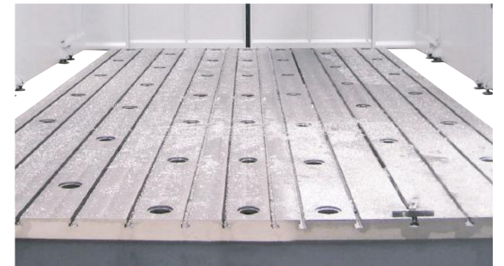
Cast iron working tables
