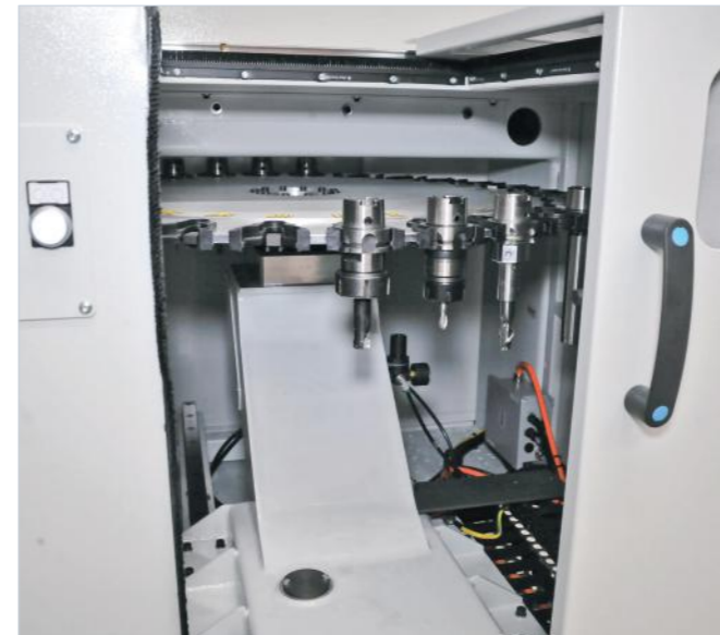
30 stations automatic rotary tool changer
