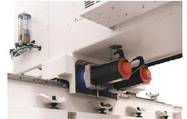
To the excellent performances of the poseidon, the concept has kinematics with two drive motors on linear axes - backlash recovery
