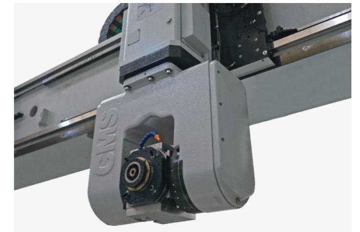
Operating unit HX5 - 20 KW
