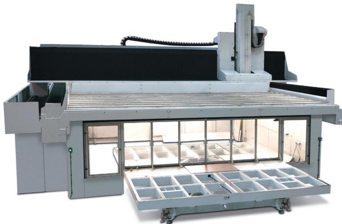
TAVOLA GIREVOLE: SEMPLIFICA IL CARICO/SCARICO FUORI DALLA MACCHINA E PERMETTE IL CICLO PENDOLARE USANDO LA COMPLETA AREA DI LAVORO
