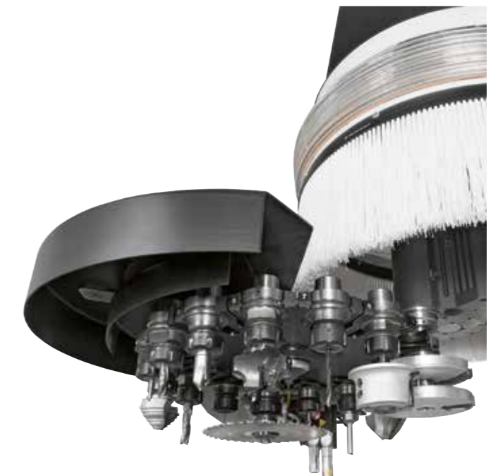
Many tools always available thanks to the R16 rear tool changer.
