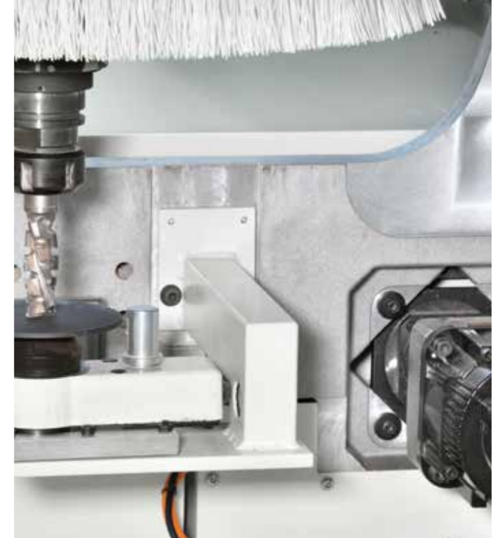
TOOL LENGTH DETECTION DEVICE Positioned on the machine base side, it allows to automatically detect the length of the tool.
