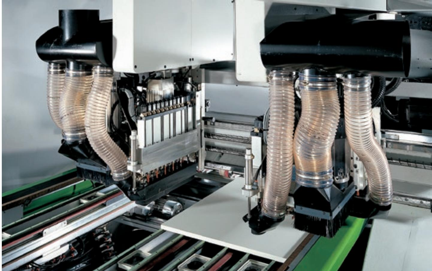
Insider FT2 is equipped with 4 machining heads fitted on two mobile carriages. Each of these units comprises 20 independent vertical spindles (10 along the X axis and 10 along the Y axis), 4 double-ended horizontal spindles (3 along the X axis and 1 along the Y axis) and is also set up to take aggregates.
