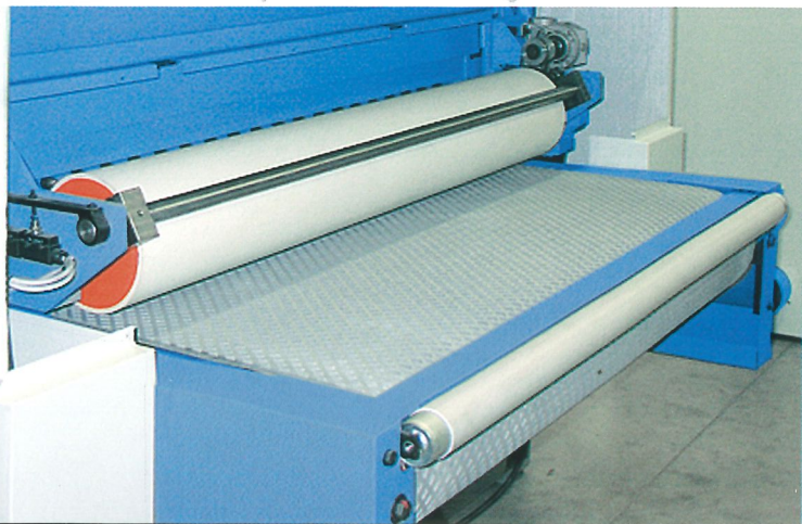
Infeed driven pressure-safety roller
