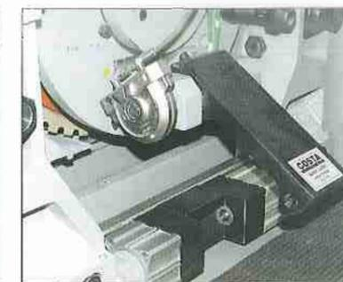
**Quick-Lock** (optional) automatic locking of working unit to the frame (for easy sanding belt change).
