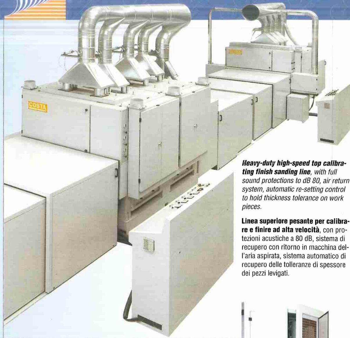
**Heavy-duty high-speed top calibrating finish sanding line**, with full sound protections to dB 80, air return system, automatic re-setting control to hold thickness tolerance on work pieces.
