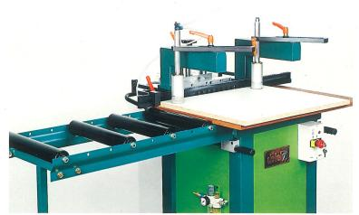
The machine is equipped with a positioning pin, place on the side-spindles, for continuous drilling. The equipment can be adjusted to meet customer's specification (variable axial distance, different number of drilling spindles etc).
