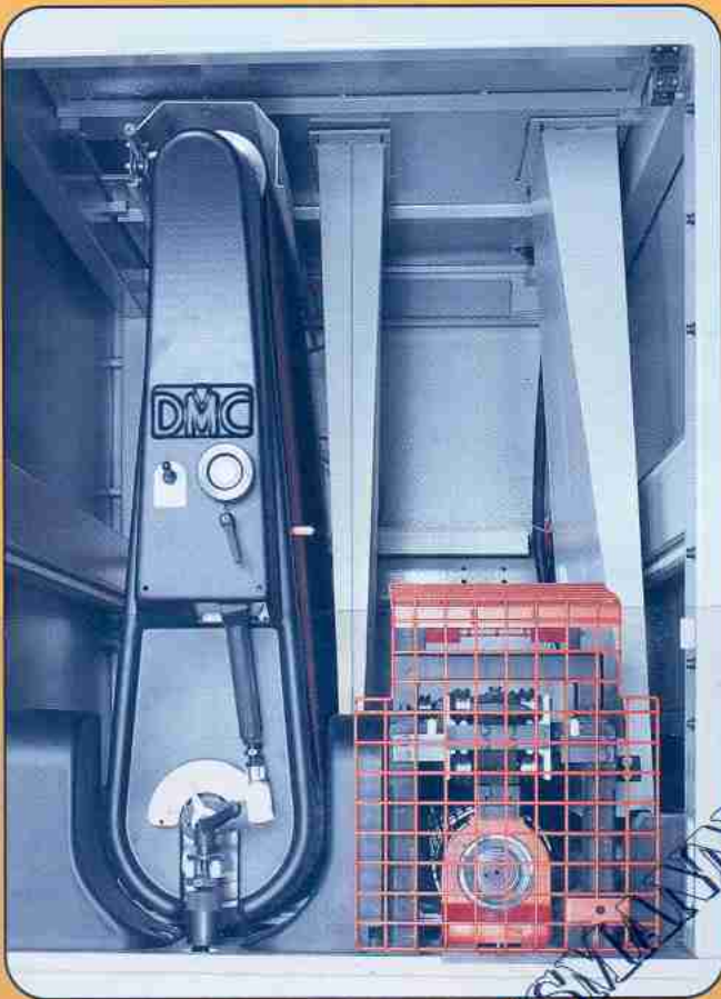
M2 CHP planer unit - Roller (250 mm) Hobelwelle CHP - Walze (250 mm)
