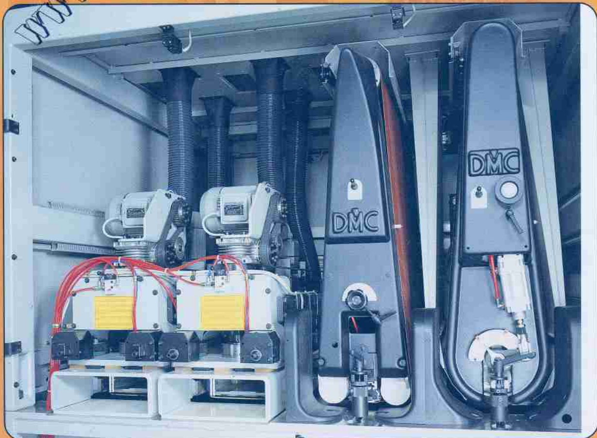
M4 Roller (250 mm) - EPICS Pad - FINESAND Pad - FINESAND Pad Walze (250 mm) - Schleifschuh EPICS - Orbitalschleifschuh FINESAND - Orbitalschleifschuh FINESAND
