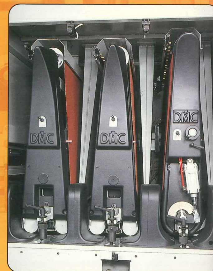
M3 Rullo (320 mm) - Pattino EPICS - Pattino EPICS Rouleau Ø 320 mm - Patin EPICS - Patin EPICS
