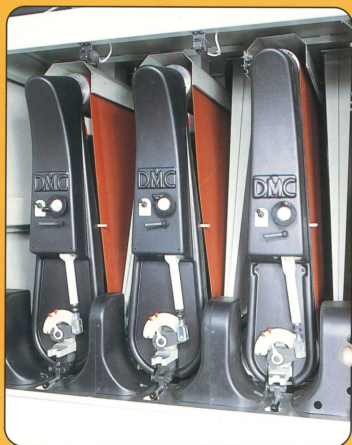
M3 Rullo (250 mm) - Rullo (320 mm) - Rullo (320 mm) Rouleau Ø 250 mm - Rouleau Ø 320 mm - Rouleau Ø 320 mm
