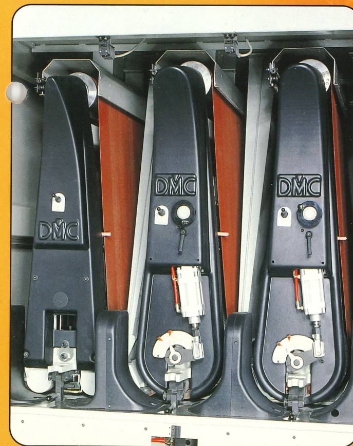
M3 Rullo (320 mm) - Rullo (320 mm) - Pattino Rouleau Ø 320 mm - Rouleau Ø 320 mm - Patin EPICS
