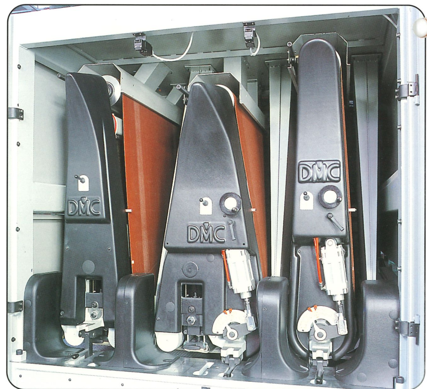
M3 Rullo (250 mm) - Combi - Pattino EPICS Rouleau Ø 250 mm - Combiné - Patin EPICS
