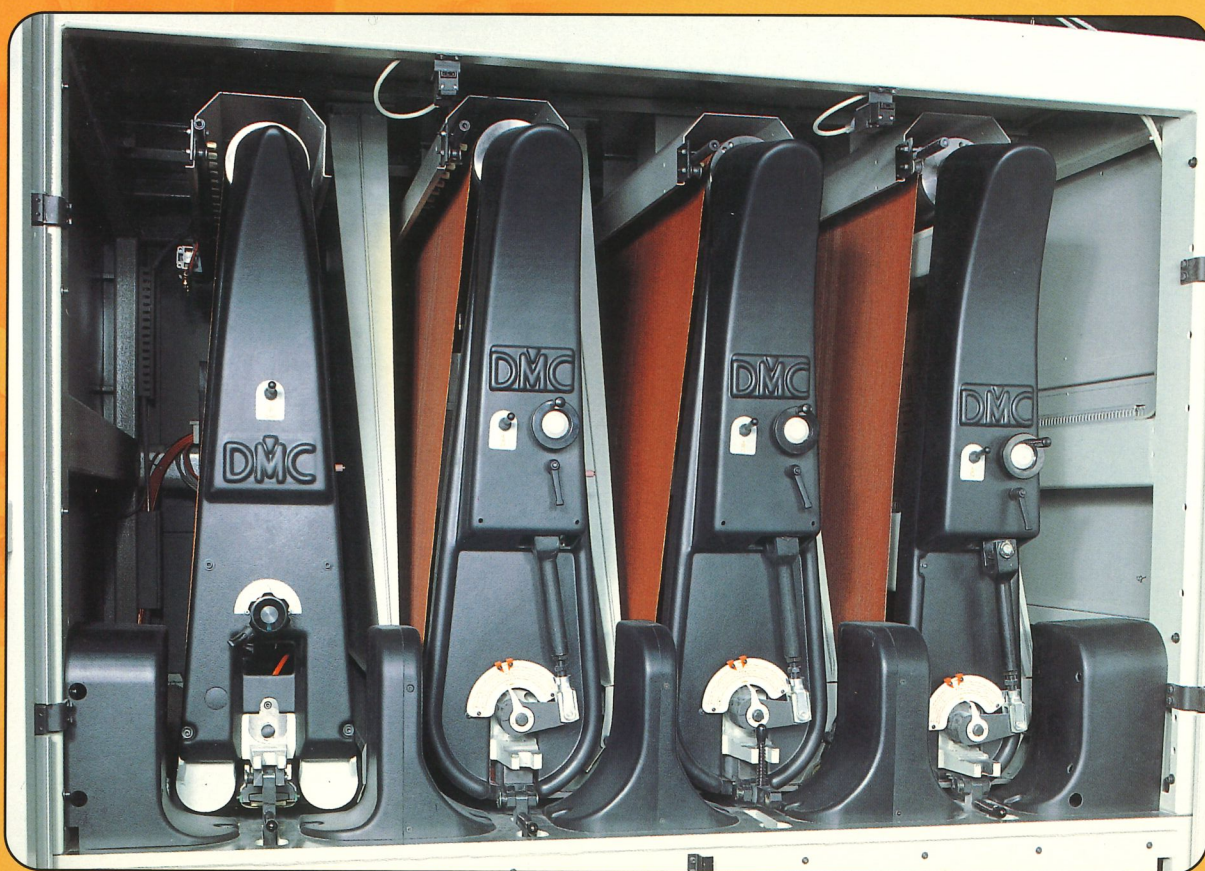
M4 Rullo (250 mm) - Rullo (250 mm) - Rullo (320 mm) - Pattino EPICS Rouleau Ø 250 mm - Rouleau Ø 250 mm - Rouleau Ø 320 mm - Patin EPICS
