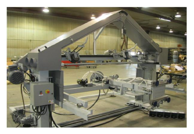
The Enclosure Box Stroke Belt Polisher includes special features designed for sanding of welded edges or polishing surfaces on steel enclosure boxes.
