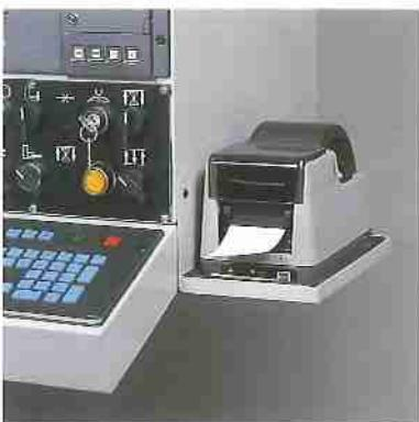
The software for the printing of labels with bar codes and its special printer are available.
