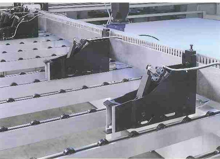
Tempus 90 with lifting table is equipped with clamps with extractable lower tooth in order to take the panel out directly from the lifting table and then, once the panels are on the wheels tables and aligned frontally, to block them.
