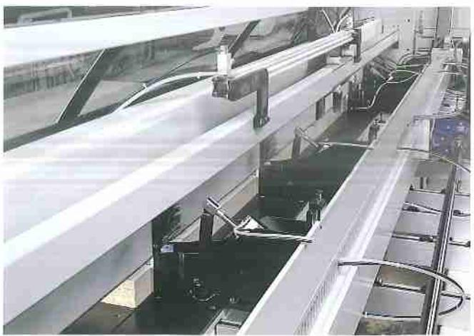
The grooved pressure beam, for the rear cut of panels, allows the clamps to reach dimensions of mm. 0; everything is extremely safe because the panels are pressed by the whole power of the main pressurer.
