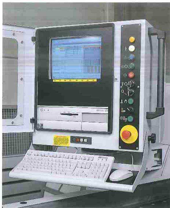
The control of the machine can be an Office PC with Windows operating system. This gives an extreme safety to the user that can always change part of the hardware that is open to all programs and to the "on line" working also for technical service via modem via the Internet.
