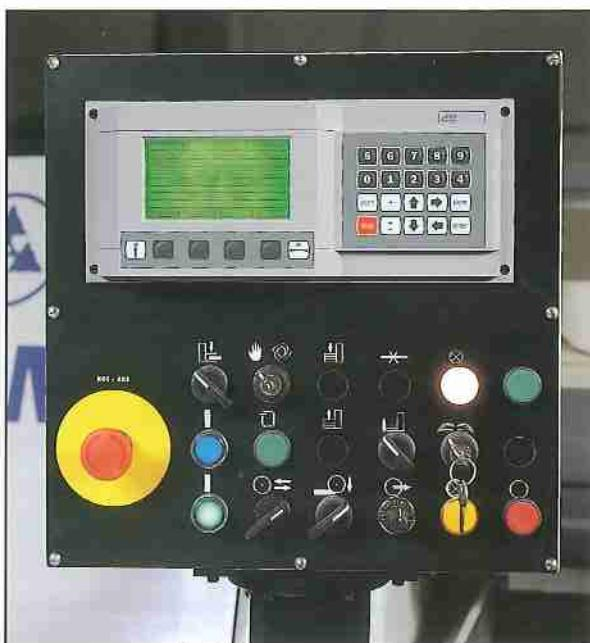
The standard electronic control with graphic video allows an easy working and reading of the programs, it is equipped with serial door for the link to other PCs in the office to load programs. The memory power is 90 complete cut patterns (with max. 30 instructions each) and continuous working of these patterns.
