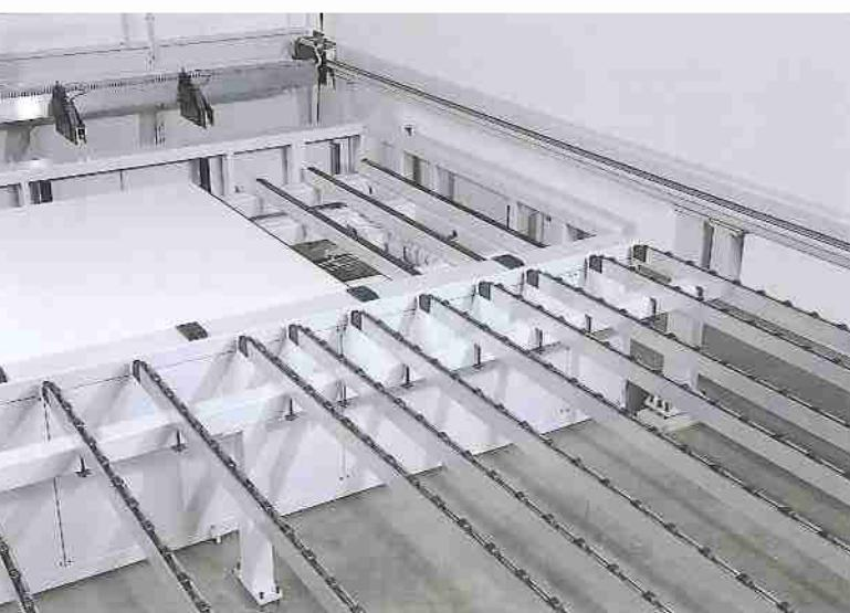
TEMPUS 90 TM is available also in the version with lifting table for automatic charge; the charge can be rear or side, by special rollers..
