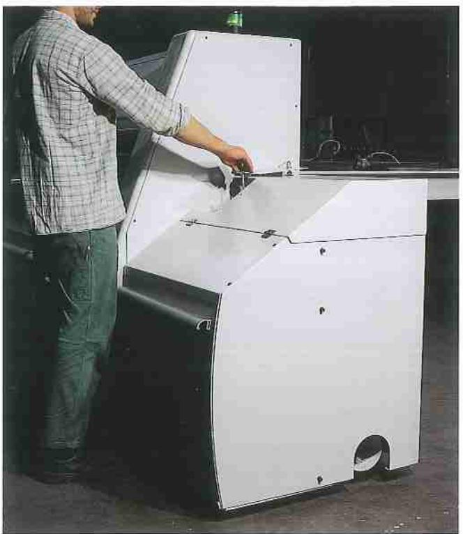
The scoring adjustment is always external when the machine is on, not to waste time on this operation.
