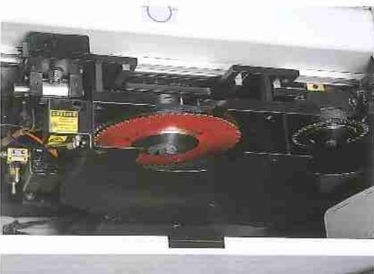
The saw carriage rolls onto two hardened and straightened guides on only one side in order to avoid tolerances of working. The scoring and blade unit lifts on prismatic guides with sliding blocks to always guarantee the maximum accuracy during the different liftings of the blade and the scoring in the postforming function. The blade motor power is transferred by a toothed belt.
