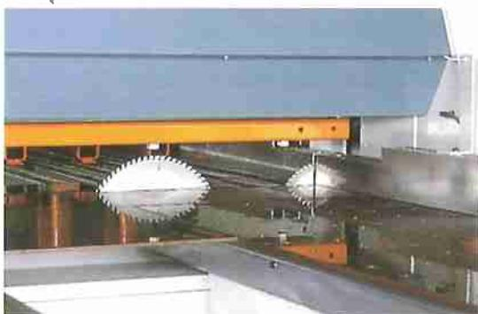
The scoring unit of the postforming version with mm. 250 blade lifts up to mm. 45 with controlled forward speed to have a perfect score and avoid chippings, thanks to the prismatic guides.
