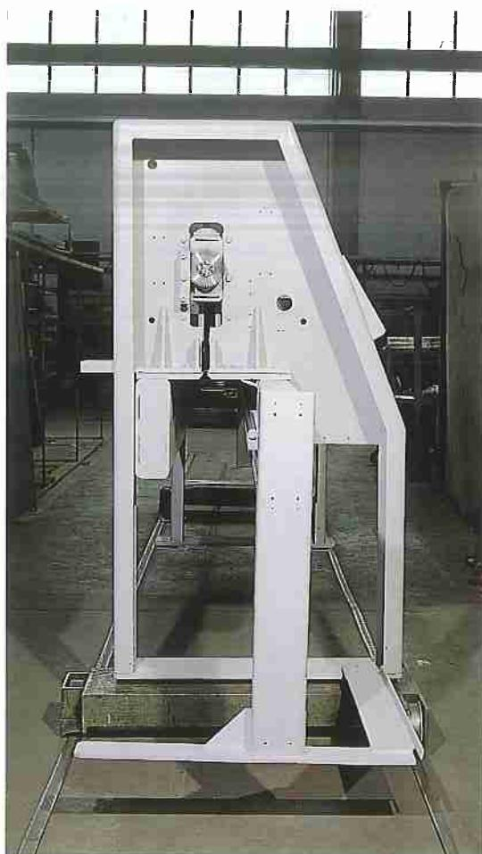
Detail of the base with the two "closed ring" juncture heads to avoid every bending which could be dangerous for the accuracy and the quality of the cut.
