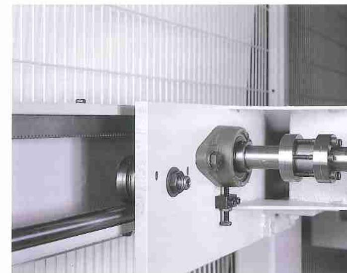
The pusher is guided by two hardened and straightened side guides and kept perfectly parallel by two bars/calibres. The pusher movement, started by brushless motor with max. speed of m. 40/min., moves onto two straightened racks and the reading is on magnetic band.
