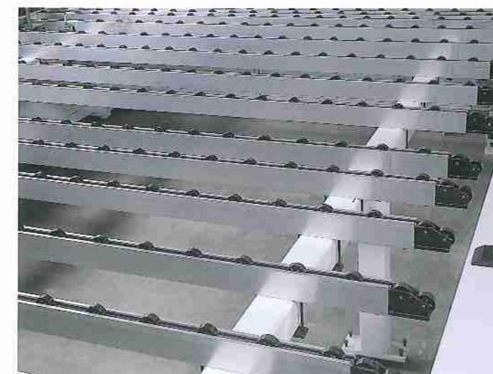
Special tables with offset wheels are available to help the panel return speed and avoid damages on their surface.
