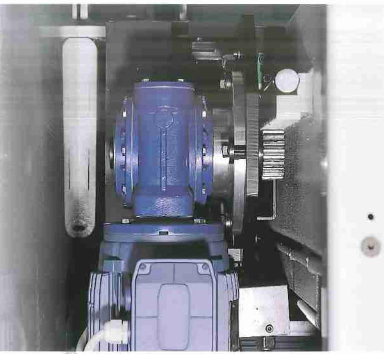
The saw carriage advances by rack to be extremely flowing and avoid dangerous vibrations made by chain and cable which could damage the quality of the cut; this way the cut is perfect.
