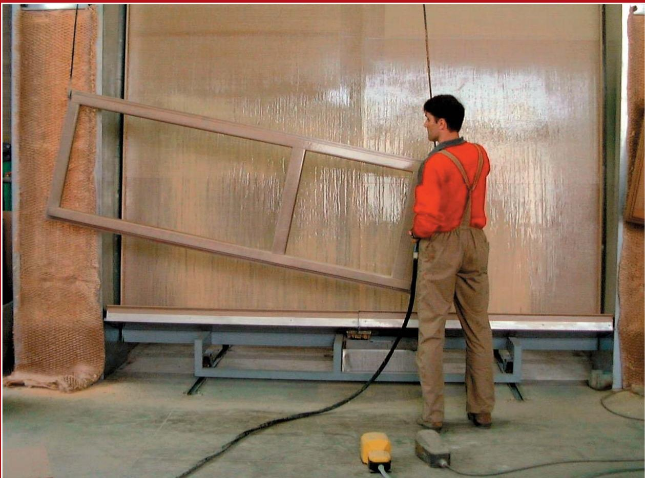
A chilled teflon-lined panel captures the paint overspray. Due to the low temperature the drying process stops and a wet film forms to keep the right viscosity of the product. The horizontal channel is chilled too, to preserve the paints characteristics until it is collected. The panels are in stainless steel isolated at the back, with labyrinthform structure inside. In the version for manual painting the panel moves back automatically to enable the bar to rotate.
