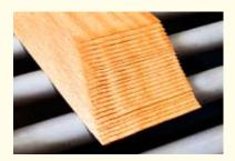
The veneer bundle is fanned both in grain and cross-grain direction directly after glue application.
