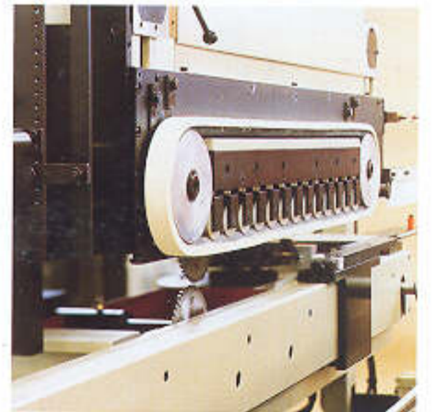
UPPER-PRESSURE SYSTEM AND FEED SYSTEM with detail of back-up blocks. Made of aluminium, hardwood or plastic material, they prevent tear-out during the profiling phase
