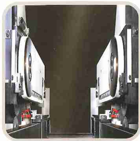
Back-up blocks. Are required to ensure no tear outs on the workpiece after profiling. The back-up blocks can be made of aluminium, hardwood or plastic material. They are mounted on the top of the feeding system.
