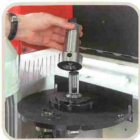
Quick tool change system. To reduce setting time of the machine and to increase the output capacity.
