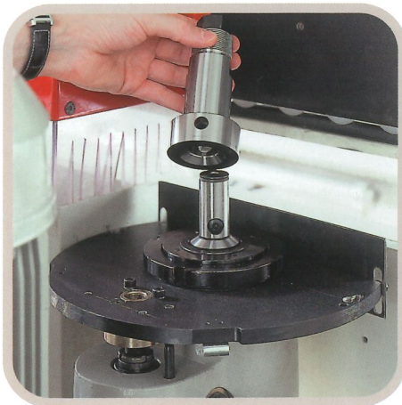
QUICK TOOL CHANGE SYSTEM to reduce the machine setting time and to increase the output capacity.
