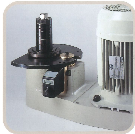
DIGITAL READ-OUT that guarantees the adjustments with centesimal tolerance.
