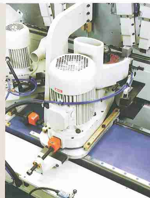
PROFILING UNIT "J-2" with back-up blocks and pneumatic chip-breaker
