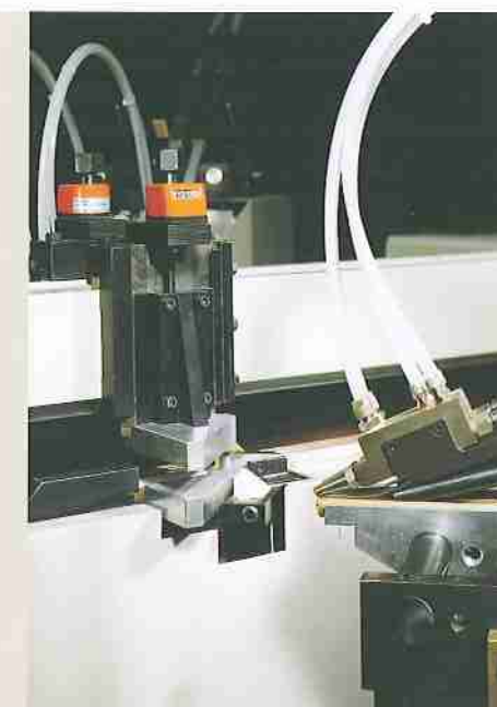
Detail view of the referencing and clamping system for working units positioned at 45° angle
