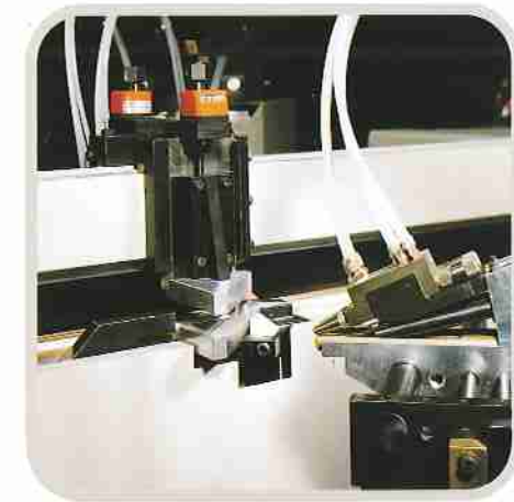
Top and bottom clamping system. This is available for all profiling-, boring-, glue injector and dowel inserting units.
