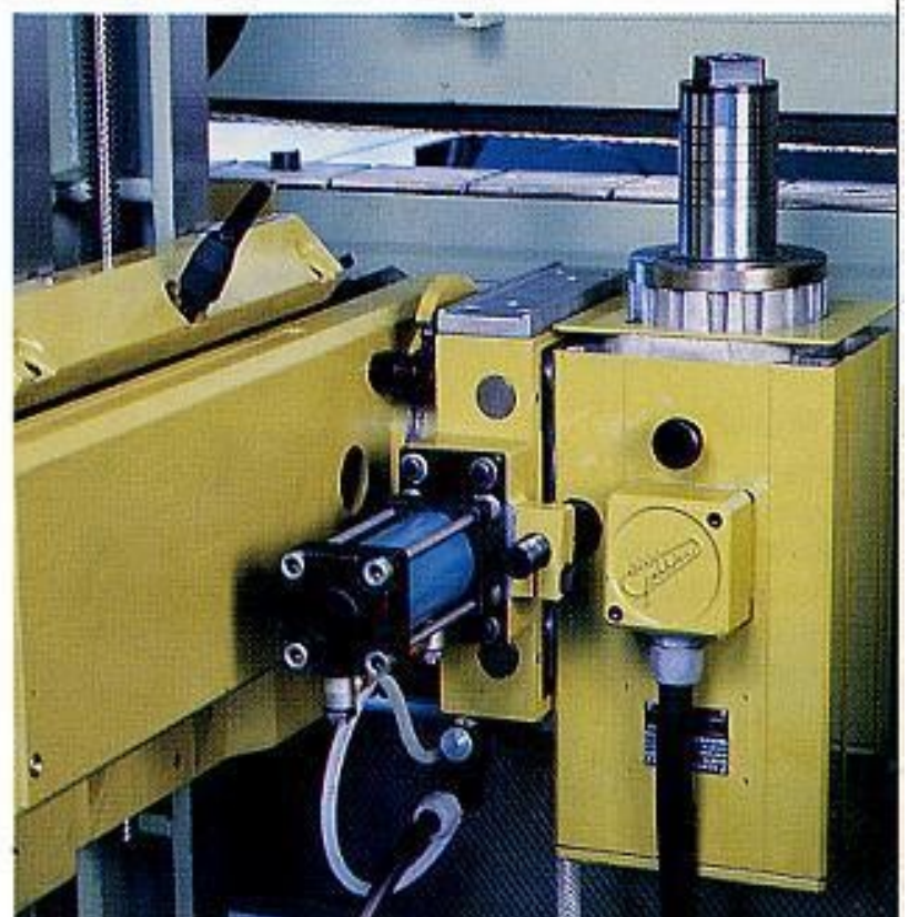
Universal milling/moulding unit with tiltable jumping device mod. 480 R
