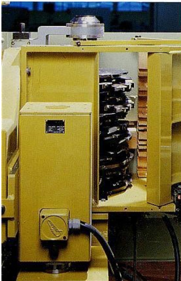
Tenoning unit with stackable tool mod. MULTIPLO 560 R with automatic chipbreaker
