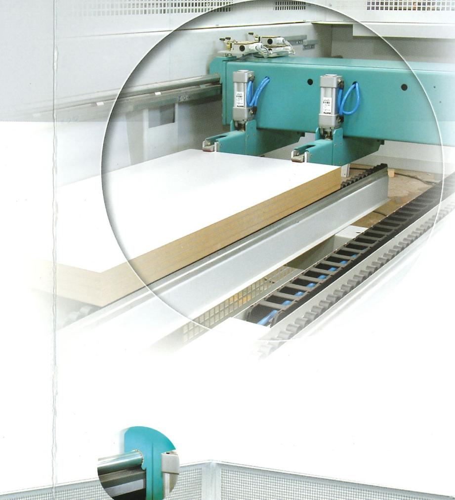
**Electronically controlled pusher** with overhead side guides equipped with pneumatic grippers.
