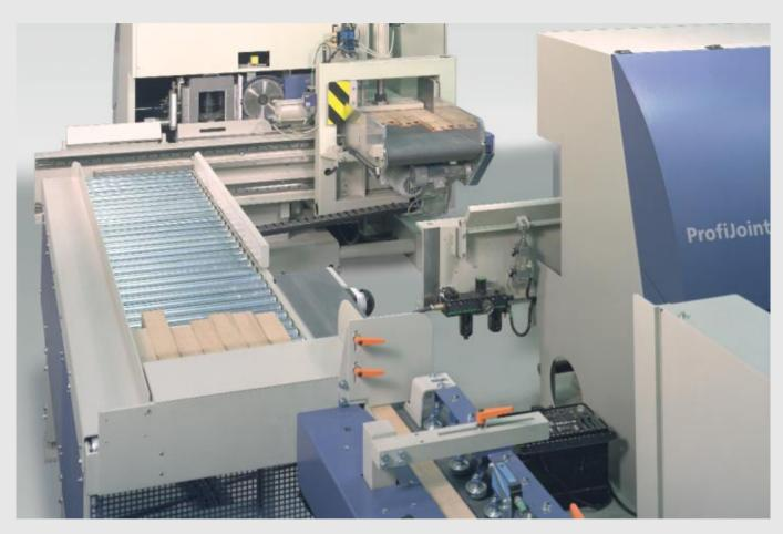
By the modular design of a finger jointing line you have the possibility to determine the degree of automation yourself. No matter whether you wish to operate a manual, a semi-automatic (including separating magazine) or a full-automatic line: Depending on the requirements GRECON recommends the right degree of automation.
