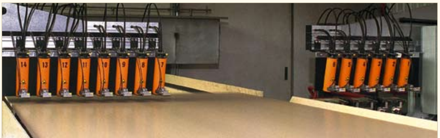
Bond Quality Measuring System UPU 3000 with ct-Frame (one side in calibration position)
