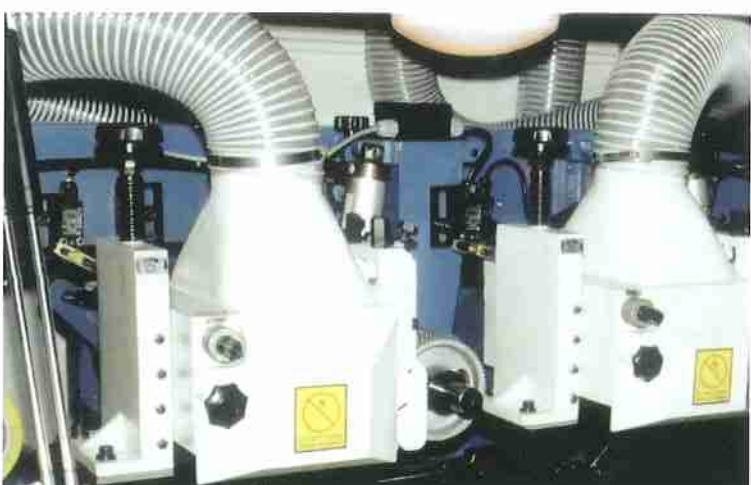
*The **NMP** series can be used for all kind of productions. The spindle sequence is – due to the NMP-unit assembly system – completely variable. Here e.g.: 2 fence side, 2 top and 2 bottom spindles. Very important for the strip-mouldings production: The top and the bottom spindle follow close after eachother. Linked from above with a solid pressure shoe !*
