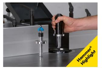
MF Spindle shaft quick change system
