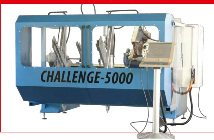
For industrial scale manufacture and to satisfy highest demands on presision and in case of extremely complexe parts, the CHALLENGE-2000 presents all technical advantages, which are characteristic for an efficient all-automatic CNC wood turning lathe. The CHALLENGE-5000 is capable of turning, milling, grooving, graving, drilling and grinding.
