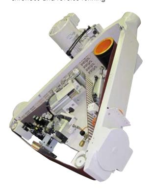
Once preset, belt tension values remain constant irrespective of different unit angle positions. This is achieved by a balanced suspension of the belt drive motor. Sanding belt speeds of 6 and 12 m/s or steplessly from 0.7 - 12 m/s.
