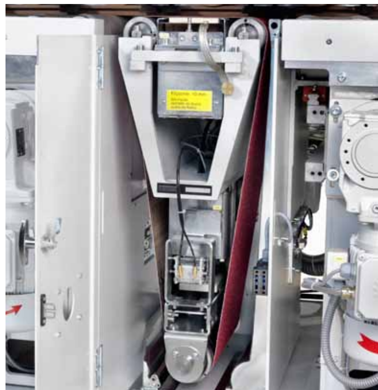
The unit L 300-U sanding from below with a sanding belt length of 1 800 mm.
