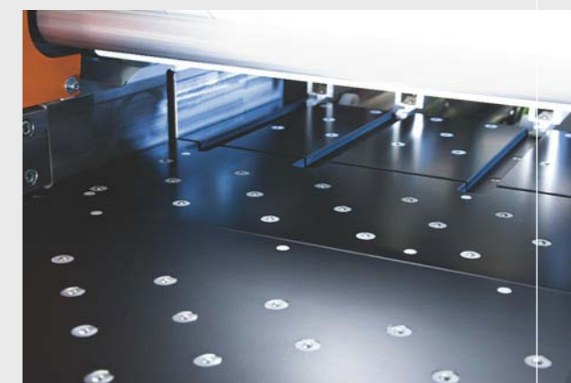
Air cushion in machine table to protect sensitive panel finishes (optional).
