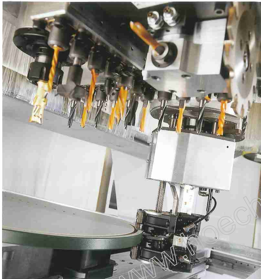
Traced combination flush trimming and scraping unit making use of the drive, C-axis and pneumatic interface
