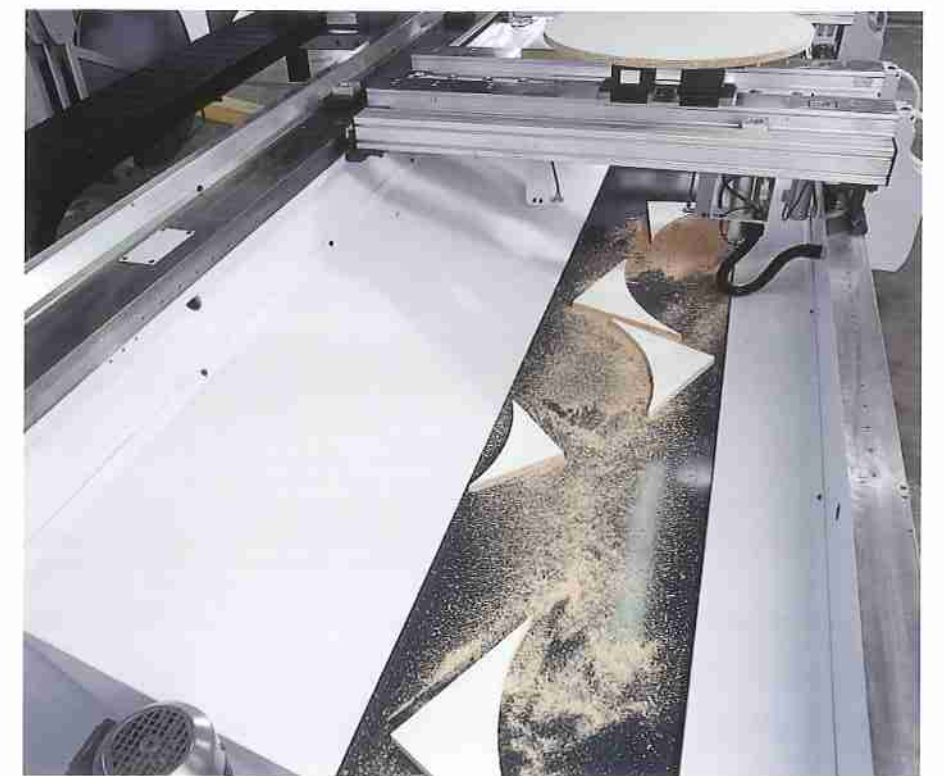
Conveyor belt for automatic waste disposal (optionally)
