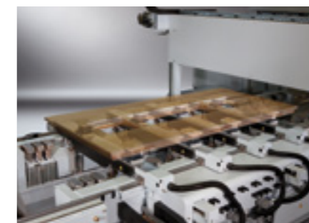
The universal clamping systems can be used simultaneously – for instance to produce front doors or semi-circular arches.
