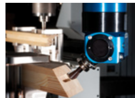
Precise mitre cuts and corner connections.
