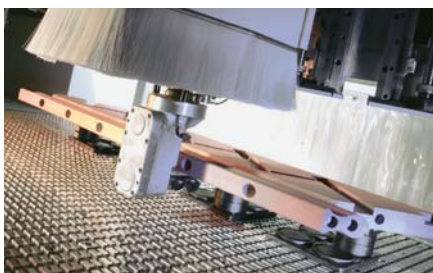
Staircase stringer processing on Flex-System
