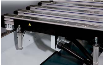
Push-off rails with two pneumatic cylinders simplify the positioning of heavy workpieces
