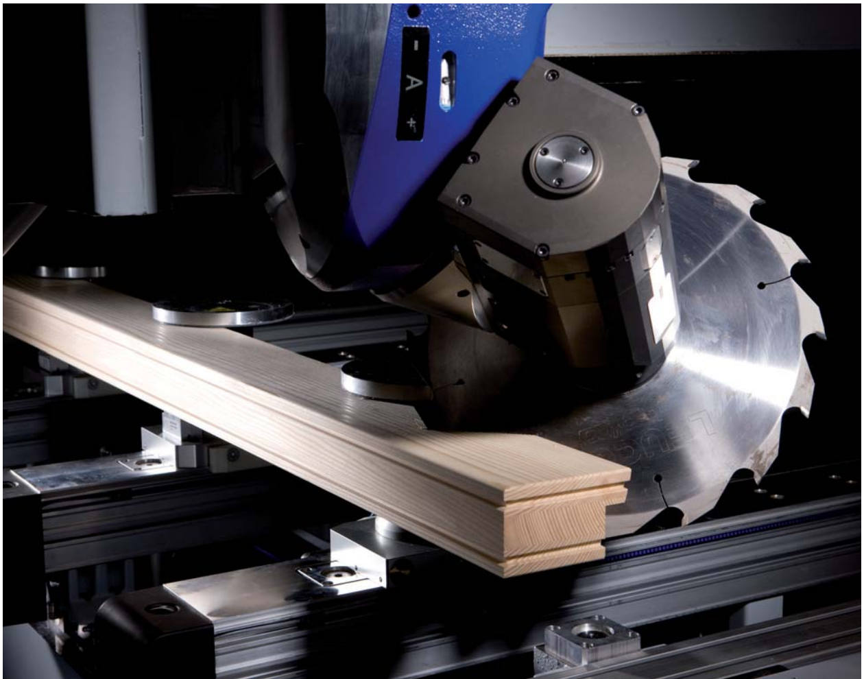
With a maximum saw blade diameter of 350 mm, even precise shift cuts for conservatory production can be executed without problems.
