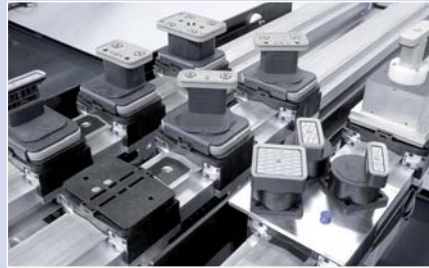
Different vacuum and pneumatic clamping elements guarantee precise processing of different workpieces and materials.
