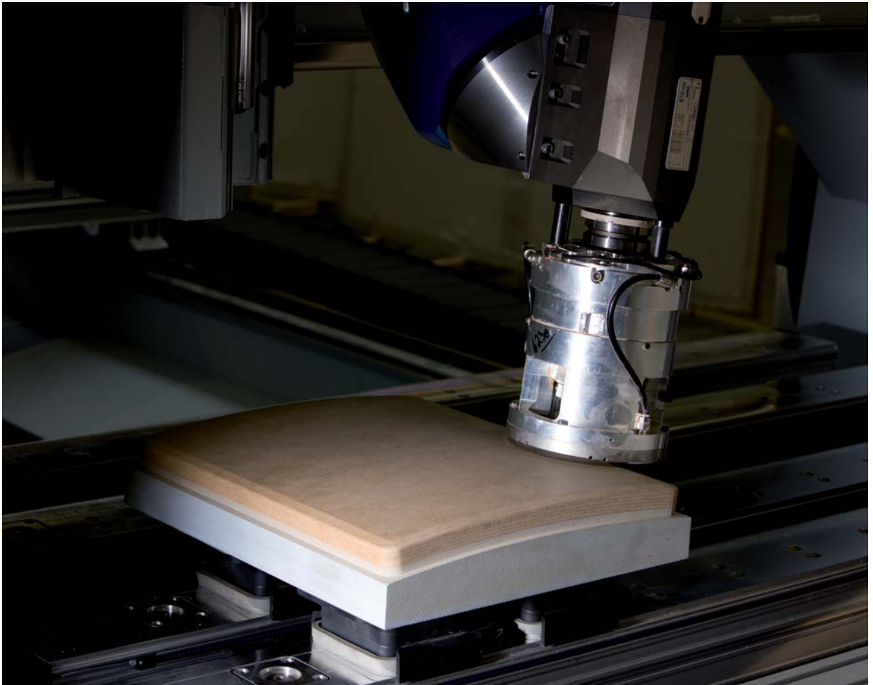
Traced trimming of curved furniture fronts with DRIVE5C+ five-axis spindle
