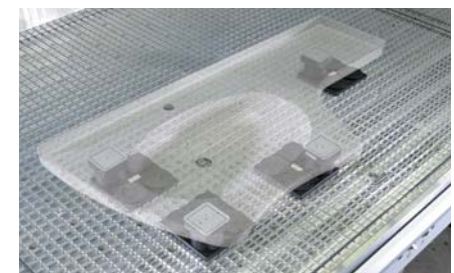
The Flex System also permits reliable fixture of curved workpieces such as washbasin units made of Corean
