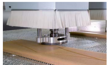
Traced trimming of furniture fronts with electronic sensoFlex tracing system
