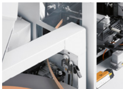
Insertion device Automatic edge infeed for quick edge changes between different rolls of material.
