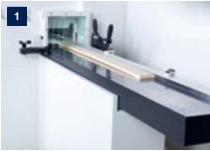
Harden chromed feeding table for long lasting service life
