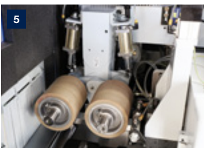
Top pressure rubber rollers for sensitive surfaces after processing (Shore hardness: 80)
