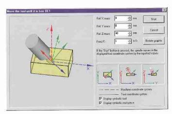
With **ECS** (Effector Coordinate System): Switchover to a coordinate system at the tool tip permits a tool to be conveniently moved clear following program interruption, e.g. in oblique boreholes or for threedimensional processing.
