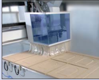
Work area of X = 3,700 mm and Y = 1,550 (Vantage 13) or Y = 1,850 mm (Vantage 15) with a processing height of 210 mm
