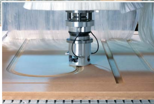
Vertical traced trimming unit for high-precision processing, e. g. of furniture fronts
