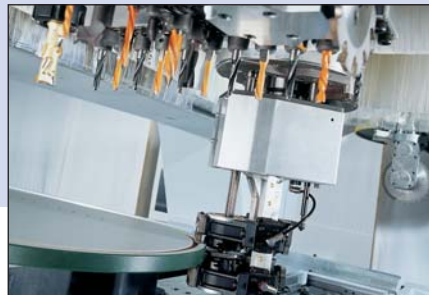
Top-quality results – the traced combi-flush trimming scraping unit which makes use of the drive system, the C axis and the pneumatic system produces stunning edge appearance. Once again, technology developed and patented by HOMAG
