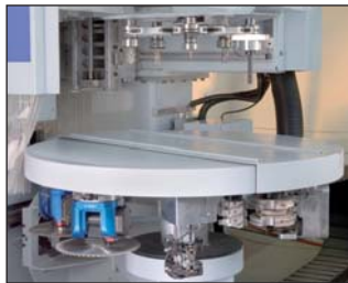
High-speed plate changer (coupled motion in the X/Y direction) with 5 slots for tools, for tool change-over during drilling operations and an additional 18-slot changer for units with a diameter of up to 200 mm
