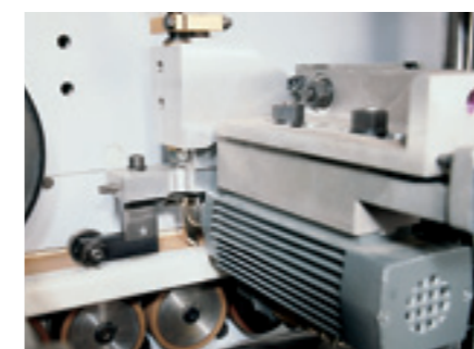
V-groove trimming unit for U-profiles for trimming a decorative groove in the cover layer or relief trimming of the laminate for parts with build-up edges
