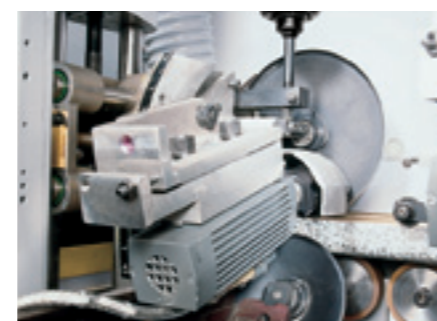
Trimming unit from above for L-profiles for flush or chamfer trimming of the overhanging laminate
