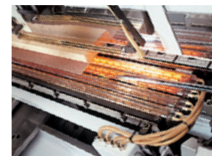
Heating and glue drying station heating lamps to thermally prepare the laminate, bending station and pressure zone
