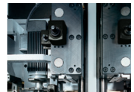
Postforming trimming unit sizing section for trimming the backing paper and the laminate overhang
