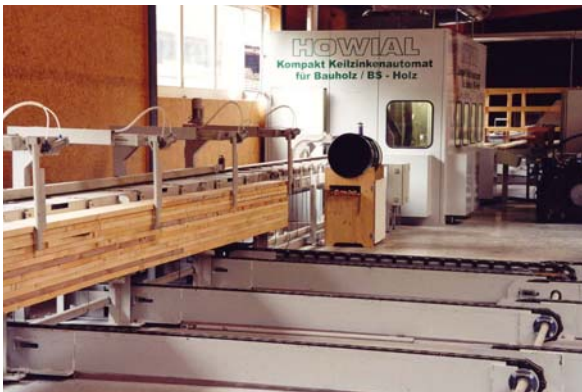
structural-timber production by a compact-finger-jointer HVP-25 and glue drying stock
