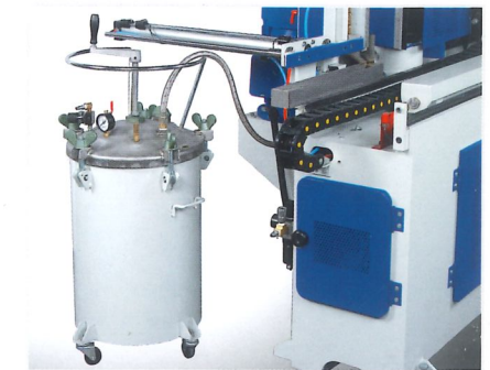
EFFICIENT GLUE MIXING TANK
