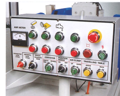
CENTRALIZED CONTROL PANEL
